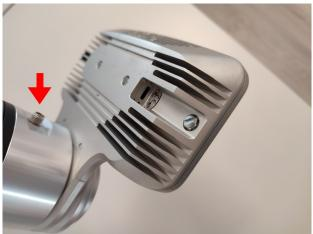
2. Mount tool adapter on top of robot adapter with the provided mounting screws.
